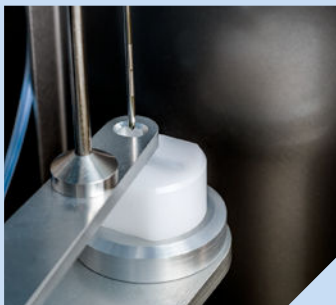
Rinsing port for cleaning the needle inside and outside
