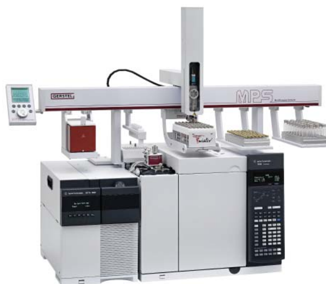
Figure 1. GC/MS system for thermal desorption of edible oils. GERSTEL Thermal Desorption Unit (TDU) mounted on a Cooled Injection System (CIS), PTV-type inlet and an Agilent GC 7890 / MSD 5977.
