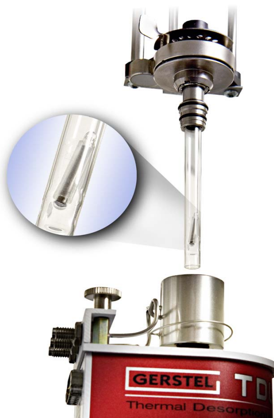
Figure 1. The GERSTEL Twister, used for stir bar sorptive extraction of drugs and pharmaceuticals from brain tissue in the work reported here.
