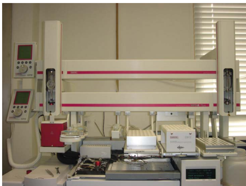
Figure 1. A picture of the dual rail GERSTEL MPS 2 with DPX automation platform. The left MPS is equipped with a 100 µL syringe for injecting eluent and derivatizing reagents, and the right MPS is equipped with a 2.5 mL syringe for performing DPX extractions.
